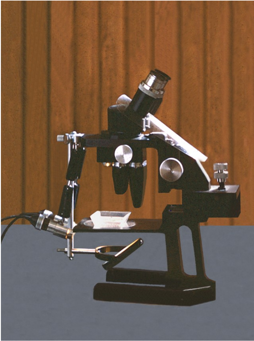
Picture 8 (1960). The Leitz UK IV. The y-movement knobs are on the right hand side.
