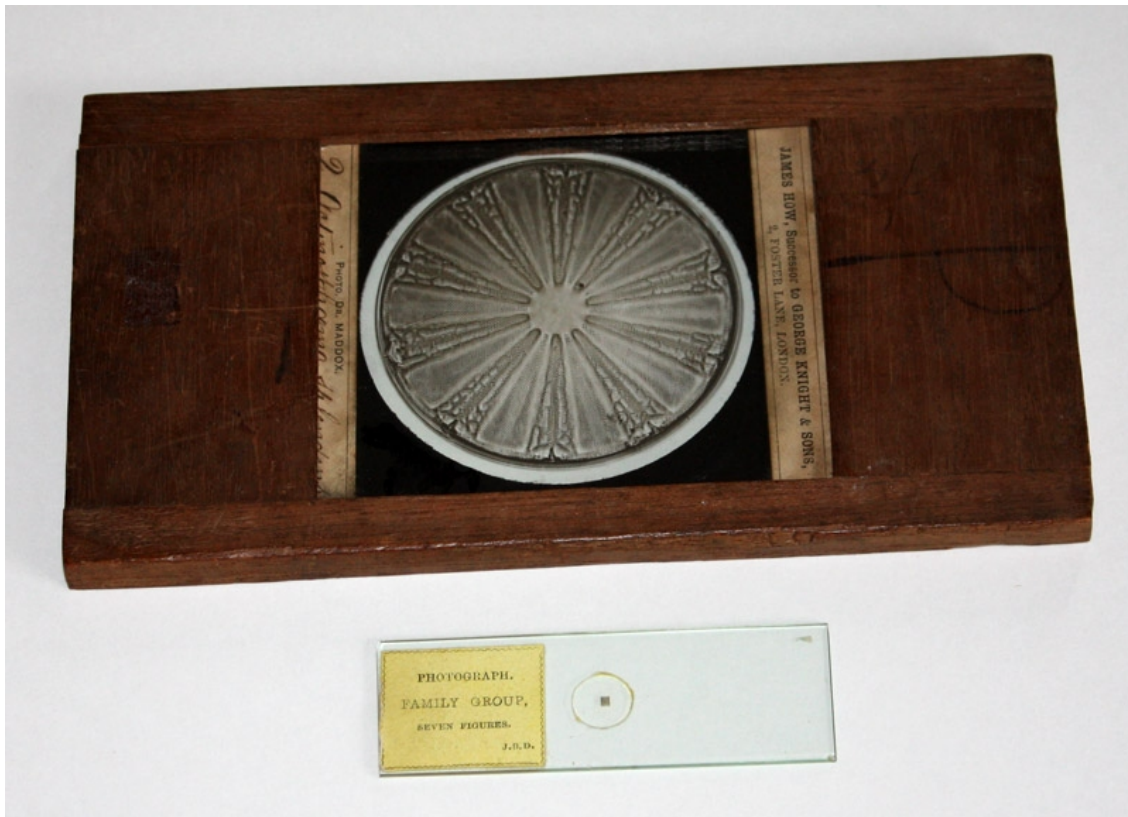
Figure 1. The two extremes of the union of microscopy and photography: a lantern slide of a photomicrograph by R.L. Maddox alongside a microscope slide of a microphotograph by J.B. Dancer. Both date from the mid-1800s.
