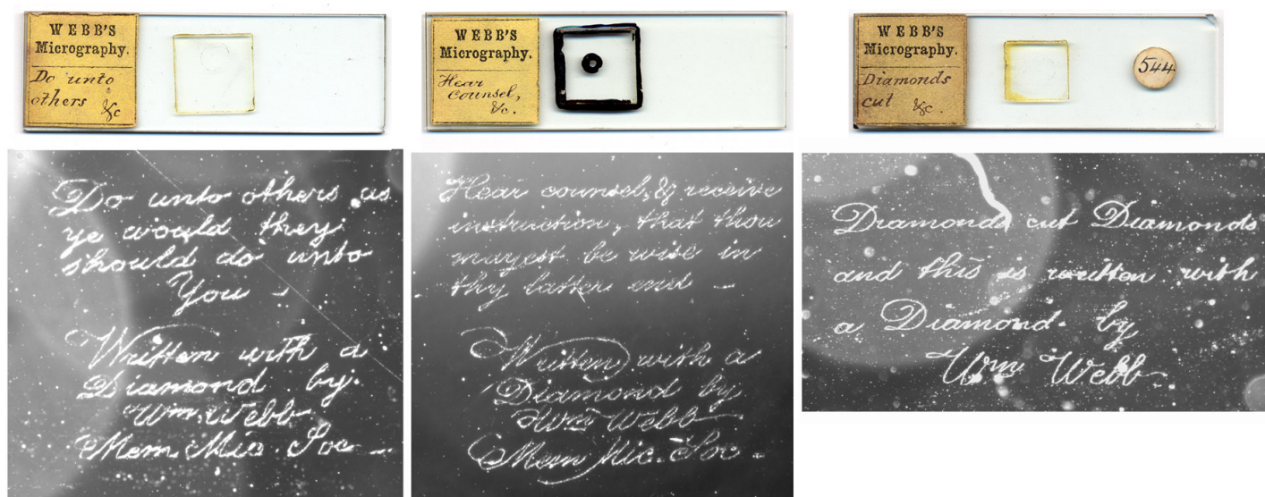
Figure 1. Examples of micro-engravings produced by William Webb, with his own trade labels. Images of the engravings were photographed using darkfield illumination.
