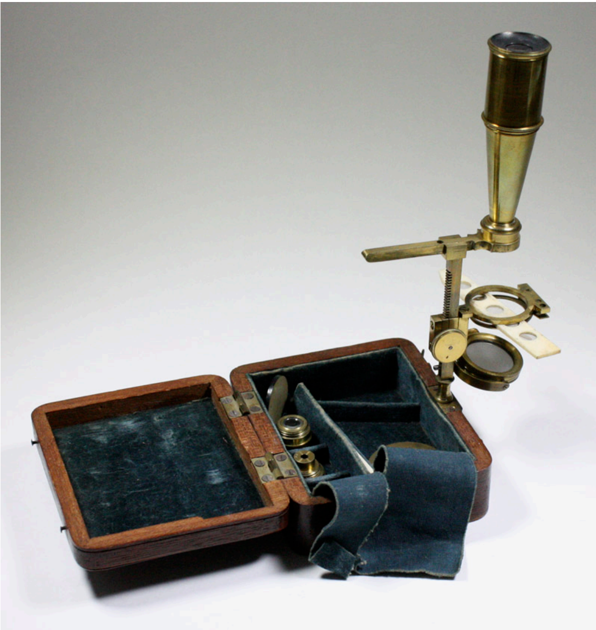
Figure 1. A ca. 1828 example of the original, small, box-mounted microscope designed by Charles Gould.
