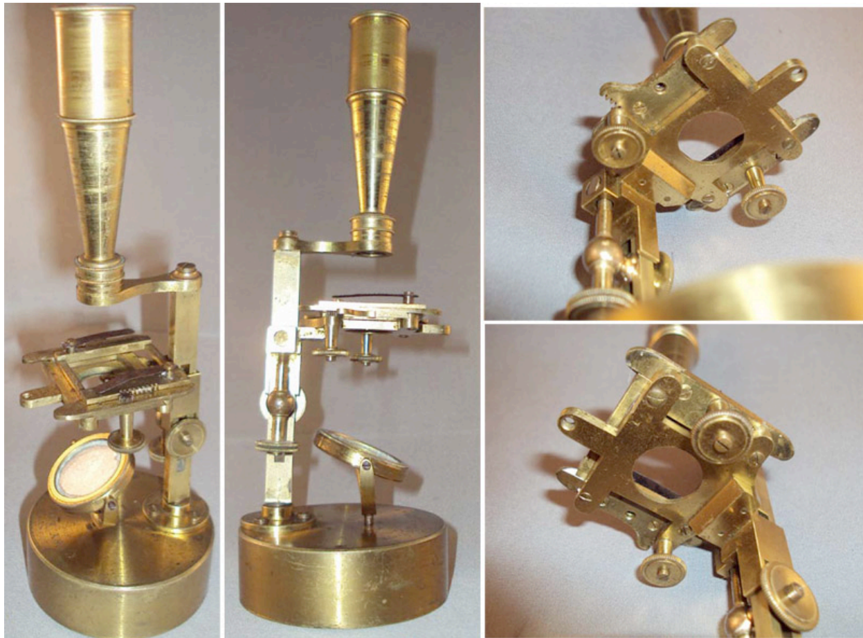
Figure 17. An example of a Cary microscope with Gould's adjusting stage. Adapted, with permission, from http://www.microscope-antiques.com/carymech.html
