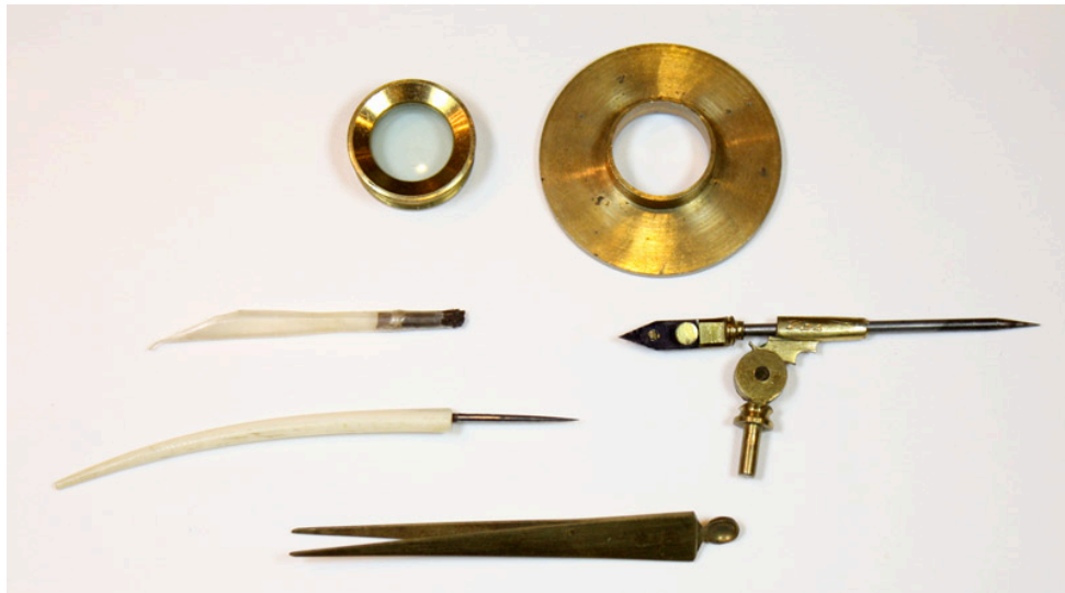
Figure 11. Accessories that accompanied the microscope shown in Figure 1 at the time of acquisition, and were listed by Gould as accompanying the microscopes he produced. Clockwise from top left: live box, stage mount for the live box, steel-pointed stage forceps, brass forceps with spoon at one end, a dissecting needle with ivory handle, and a brush made of fine hairs inserted into the end of a feather shaft. Originally, a small knife with a handle like that of the needle would also have been included.
