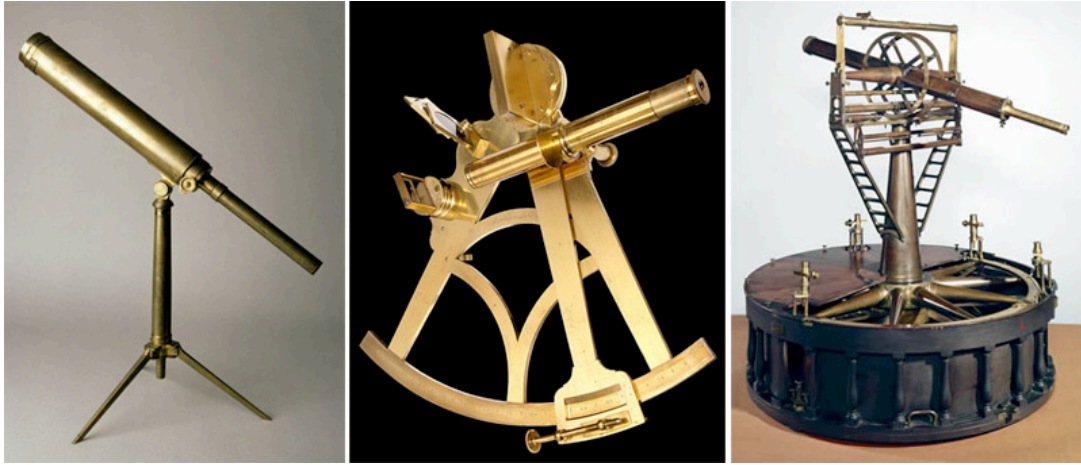
Figure 31. Scientific apparatus produced by Jesse Ramsden, with whom William Cary served his apprenticeship. Left to right: refracting telescope (from http://www.hps.cam.ac.uk/whipple/explore/astronomy/twotelescopes/ ); sextant (from http://www.mhs.ox.ac.uk/sis25/image.php?id=45 ); theodolite (from http://www.ramsden.info/Ramsden/Ramsdens/JesseRamsden.htm ).
