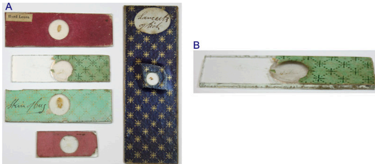
Figure 15. Another contribution of Charles Gould to the evolution of microscope slide-making. (A) The four small slides on the left were made according to what Thomas Gill described as “Mr. C. Gould’s Mode” of slide making. The specimens were dry-mounted between a mica cover slip and a glass slide. Paper was glued on top, to help hold down the cover slip and prevent it from being dislodged. The torn paper on the damaged slide reveals the mica cover slip. The top red-papered slide with the printed label was retailed by Andrew Pritchard (it is part of a set that was acquired in a case that is embossed with Pritchard’s name and address). The two slides with pale green papers with star prints were produced by professional slide-maker James W. Bond. The lower, small slide is an early test slide of butterfly scales, possibly retailed by Cary. A later, balsam-mounted 1x3 inch slide by Bond is shown for size comparison. (B) An enlarged, oblique view of the damaged J.W. Bond slide. All of these slides have paper coverings on the top only, as Gill described for Gould’s technique. Cut edges of the glass slides were left rough.
