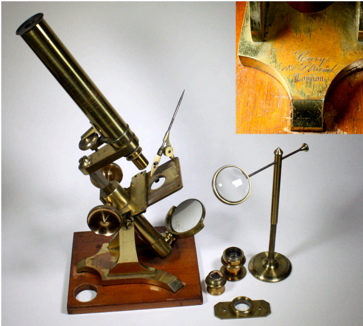
Figure 21. A Society of Arts-style microscope from Cary. The base is engraved "Cary", and so likely dates from either before Charlotte Gould and Henry Porter renamed the business ca. 1859, or after Porter returned the name to "Cary" ca. 1876. Accessories included with the instrument in its mahogany case were polarizing lenses, live box, stage forceps and "bull's eye" condenser.
