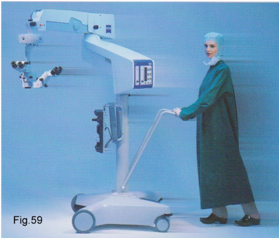
Fig. 59 Opmi VISU 200 for ophthalmic surgery (1998) with 2° and 6° coaxial illumination and with 0° assistant's microscope and x-y coupling. All settings for brightness, magnification, motor speed etc. can be stored and recalled. Automatic lamp change in case of failure.
