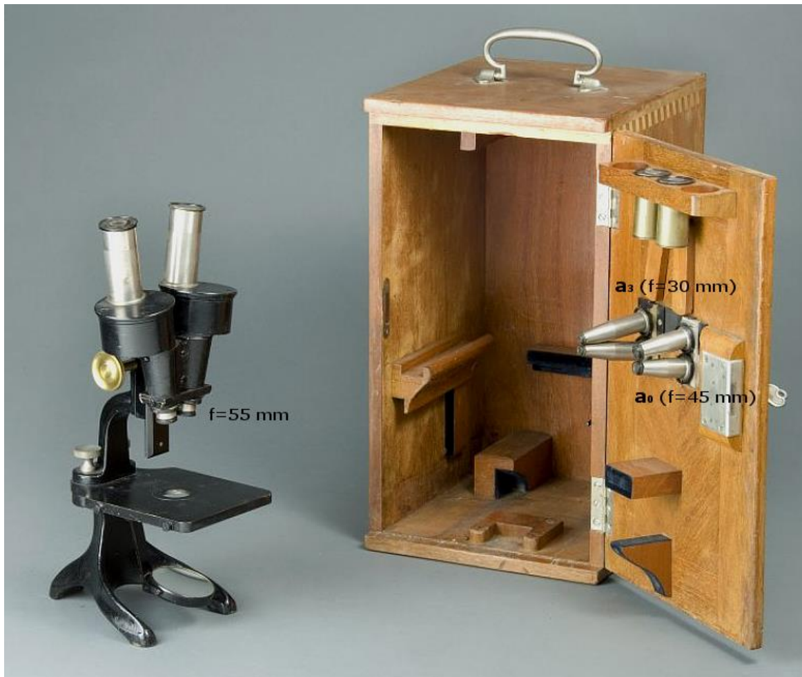
Fig. 99 Stand X a and its Box in 1910 (Courtesy Collection of Historical Scientific Instruments, Harvard University), Objective Pairs Noted by the Authors.
