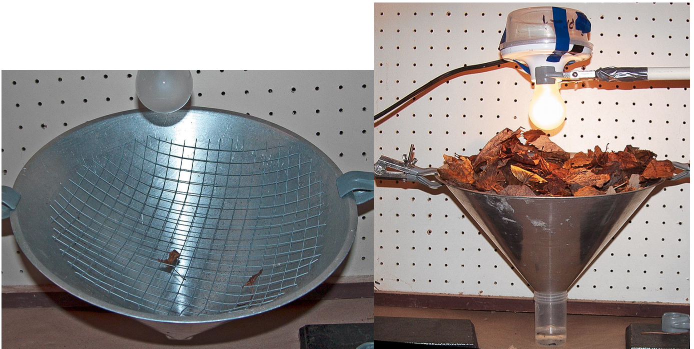
Fig. 1. Funnel with screen mesh (left); with litter sample, alcohol vial, heat/light source (right)
