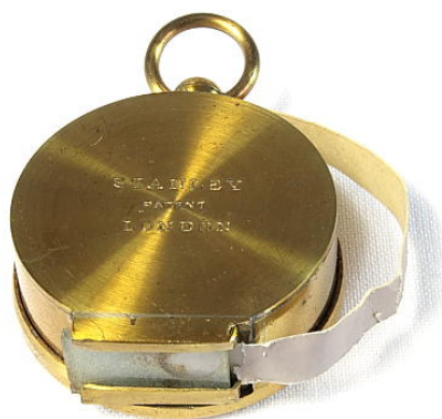
Figure 3. An actinometer produced by Stanley, from the design patented by Stanley and Sarjeant. It is roughly the size of a pocket watch, and was intended to be similarly worn on a chain.
