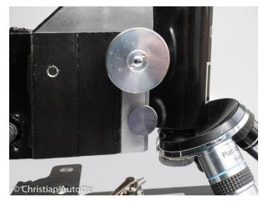
An extra screw added under the coarse focus to lock it in place
