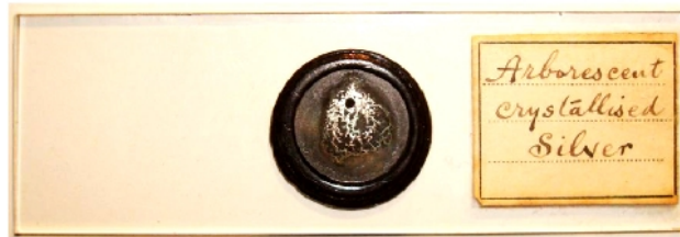
Figure 6. An Ebbage preparation of crystallized silver, prepared as described in The English Mechanic and World of Science , 1891. Note the hole in the crystals where Ebbage had placed the copper wire.
